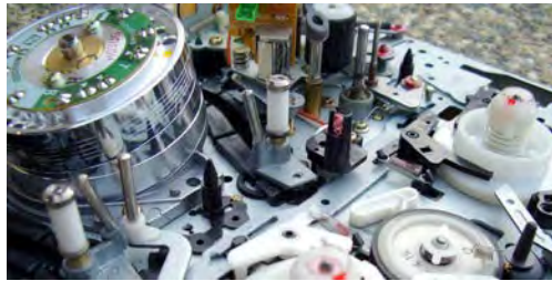
Figure 23.8 Recording and playback heads used with audio and video magnetic tapes. (credit: Steve Jurvetson)
