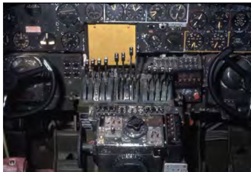
Figure 31.2 The dials of this World War II aircraft glow in the dark, because they are painted with radium-doped phosphorescent paint. It is a poignant reminder of the dual nature of radiation. Although radium paint dials are conveniently visible day and night, they emit radon, a radioactive gas that is hazardous and is not directly sensed. (credit: U.S. Air Force Photo)
