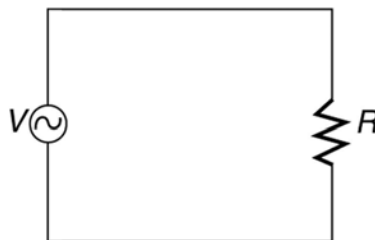
Figure 23.31 Schematic of a simple AC circuit with a voltage source and a single appliance represented by the resistance R . There are no safety features in this circuit.
